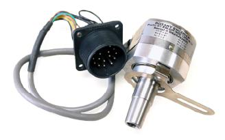
Our ST-EN-DR-ROD is a drop-in replacement for the Heidenhain ROD320 encoder. It is designed to provide precision feedback control for Siemens 1FT series Simodrive motors. It features a tapered shaft and custom flex mount. It comes in many line counts; 2,000,2,500, or 5,000 CPR,9" of cable and a 17 pin connector with the correct Heidenhain pinout.
